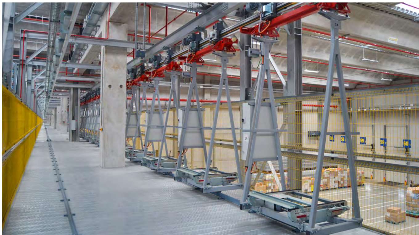
A monorail suspension system conveys the pallets within the extended Almarai production complex. 40 monorail trolleys are in use in the logistics center alone.
