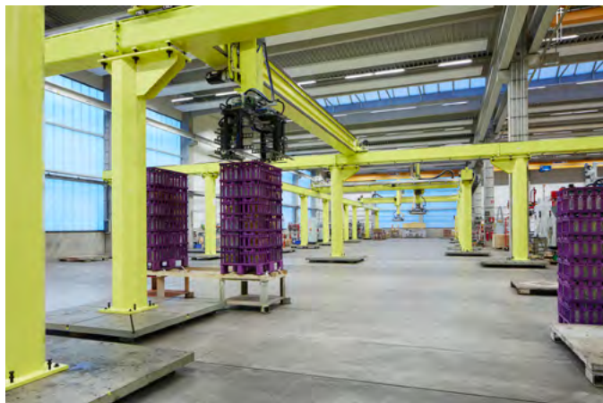
The KUKA robot is able to pick up an entire layer of drink cartons using its mechanical gripper.
